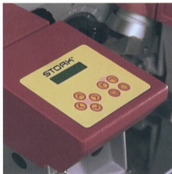
Each printing position will have a new control panel with touch keys.
